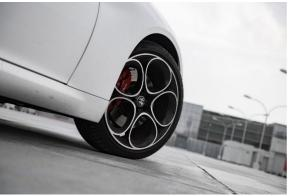
Telephone-dial style rims are de rigueur for Alfa Romeo, and the Giulia Veloce smartly wears its 19-inch items with AR-mark staggered Pirelli P Zero tyres, with 225/40 R19 in front and 255/35 R19 at the back.
