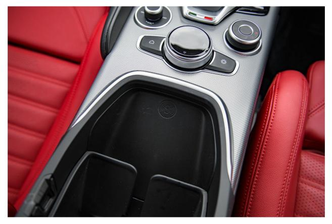
The wireless charger for mobile phones is also situated just below and ahead of the centre armrest, which is a convenient spot to simply drop one's phone into.
