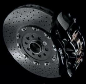
Carbon-ceramic brake disks Black Brake Calipers (optional)
